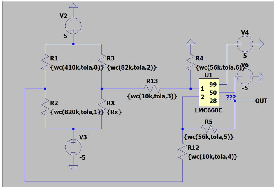
Figure 8.3.1: Wheatstone Bridge Circuit
