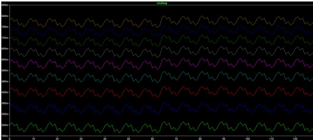
Figure 8.3.2: Wheatstone Bridge Circuit with tolerance of 1%
