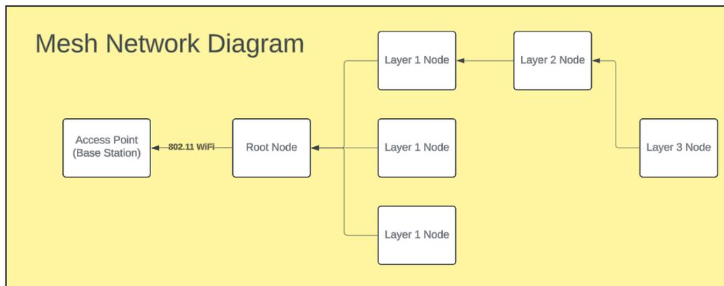
Figure 4.5.2: Mesh Network Design
