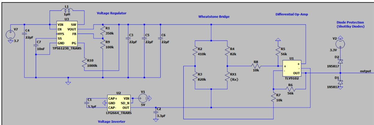
Figure 6.1.1: Unified Circuit Design
