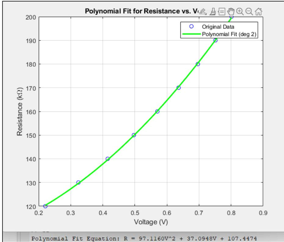
Figure 5.8.1: Voltage vs Resistance Graph
