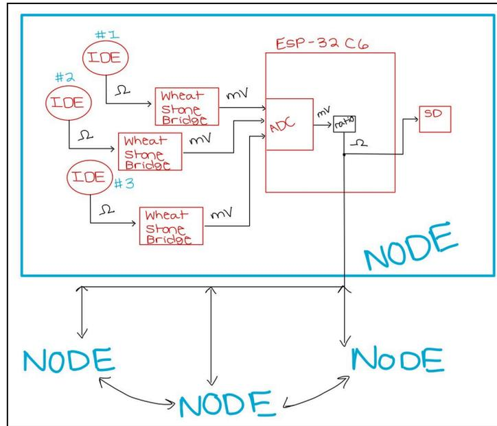
Figure 4.3.2: Block diagram of the sensor data path
