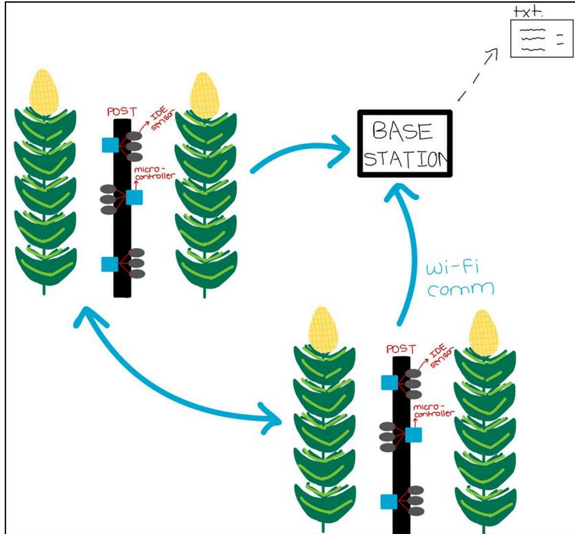
Figure 4.3.1: Simplified overview of the communication system
